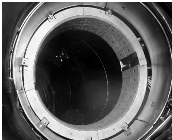
Fig. 1. BSTDG coated with SiC gradient coating as new limiter in HT-7.
